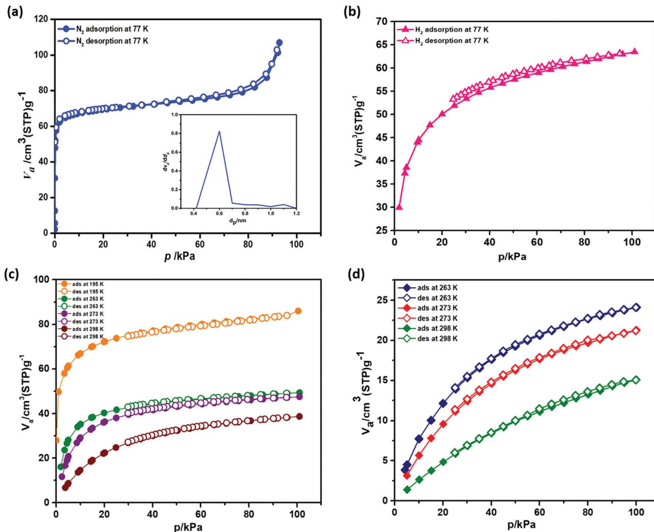
Fig. 4 Gas sorption of Zn-CBS: (a) N<sub>2</sub> sorption isotherm and pore size distribution; (b) H<sub>2</sub> sorption isotherm at 77 K; (c) CO<sub>2</sub> sorption isotherms at 195 K, 263 K, 273 K, and 298 K; (d) CH<sub>4</sub> sorption isotherms at 263 K, 273 K and 298 K.
