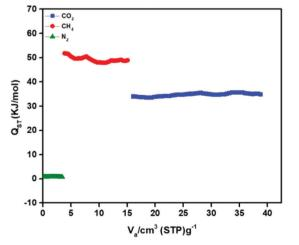
Fig. 5 Isosteric heat of adsorption ( $Q_{st}$ ) for CO<sub>2</sub>, CH<sub>4</sub> and N<sub>2</sub> using experimental isotherm data of Zn-CBS at 263 K, 273 K and 298 K.
