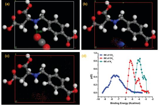
Fig. 8 CBMC simulation: (a) interaction and distance between  $CO_2$  molecules and  $H_3(p-2,4-cbs)$  present as a trianion in **Zn-CBS** at 298 K; probability density of (b)  $CH_4$  and (c)  $N_2$  at 298 K; (d) binding energy of  $CO_2$ ,  $CH_4$ , and  $N_2$ .
