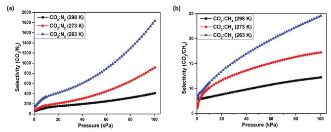
Fig. 7 Separation selectivity of Zn-CBS at 263 K, 273 K, and 298 K predicted by IAST for (a) CO<sub>2</sub>/N<sub>2</sub> (15/85); and (b) CO<sub>2</sub>/CH<sub>4</sub> (50/50).
