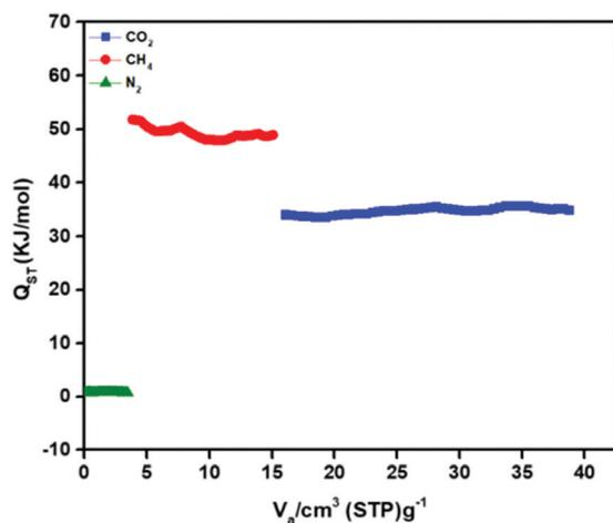
Fig. 5 Isosteric heat of adsorption ( $Q_{st}$ ) for CO<sub>2</sub>, CH<sub>4</sub> and N<sub>2</sub> using experimental isotherm data of Zn-CBS at 263 K, 273 K and 298 K.
