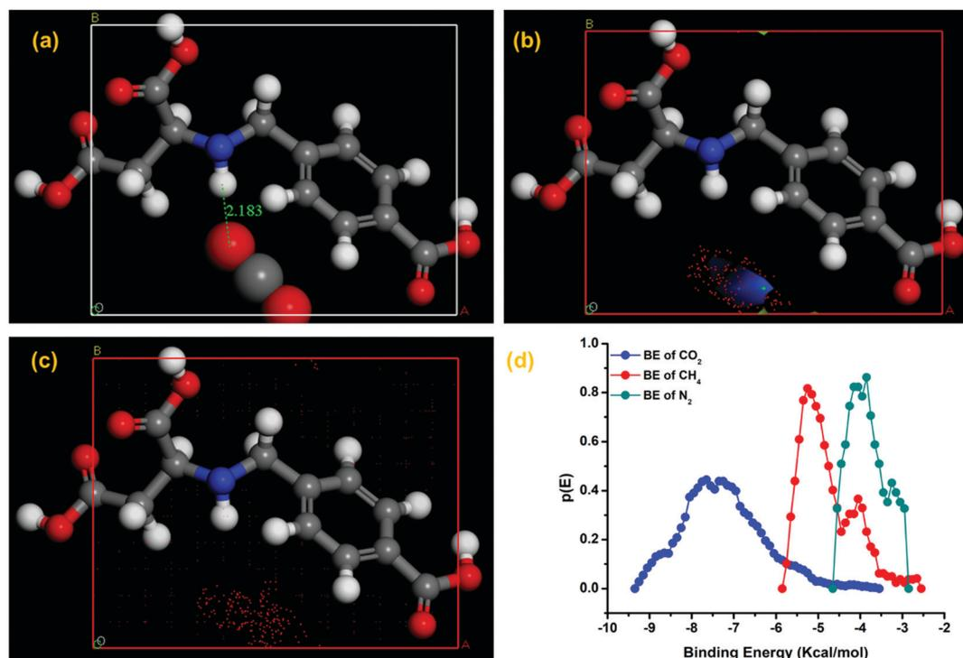
Fig. 8 CBMC simulation: (a) interaction and distance between  $\text{CO}_2$  molecules and  $\text{H}_3(\text{b-2,4-cbs})$  present as a trianion in **Zn-CBS** at 298 K; probability density of (b)  $\text{CH}_4$  and (c)  $\text{N}_2$  at 298 K; (d) binding energy of  $\text{CO}_2$ ,  $\text{CH}_4$ , and  $\text{N}_2$ .
