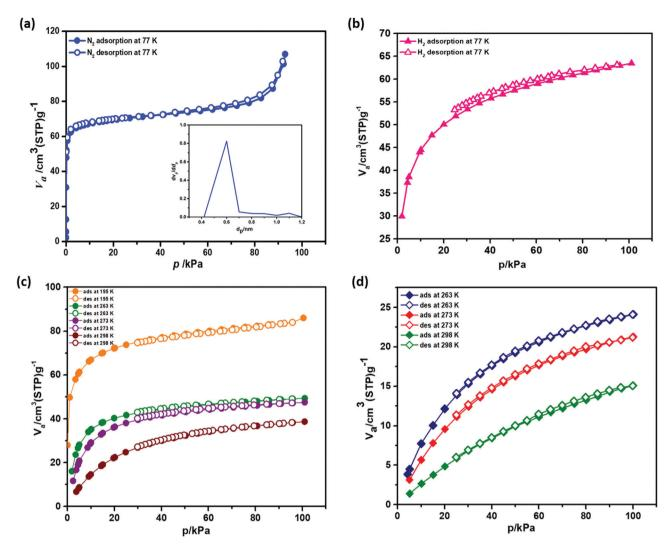
Fig. 4 Gas sorption of Zn-CBS: (a) N<sub>2</sub> sorption isotherm and pore size distribution; (b) H<sub>2</sub> sorption isotherm at 77 K; (c) CO<sub>2</sub> sorption isotherms at 195 K, 263 K, 273 K, and 298 K; (d)  $CH_4$  sorption isotherms at 263 K, 273 K and 298 K.
