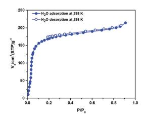
Fig. 6 Water adsorption-desorption isotherm of Zn-CBS.
