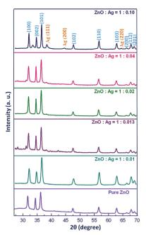
Fig. 6 X-ray diffraction patterns of pure ZnO and different sets of Ag/ZnO microstructures
