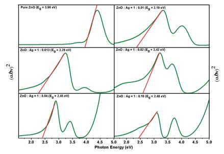
Tauc plot for the estimation of the band gap energy of pure ZnO and different sets of Ag/ZnO microstructures.
