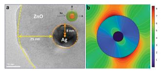
Fig. 11 (a) Representative transmission electron micrograph (set B) for parametric assignment and (b) calculation of electric field corresponding to single silver nanoparticles in Ag/ZnO microstructures through the finite element method. Inset in panel (a) shows the polarisation direction of the incident light.
