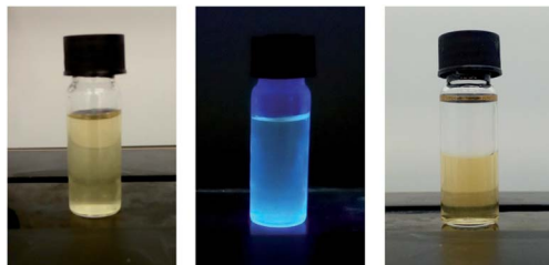
Fig. 8 Glucose-coated Si NPs in water under normal light (left) and 365 nm irradiation (middle). The right picture shows the solubility of glucose-coated Si NPs in hexane (top layer) and water (bottom layer).
