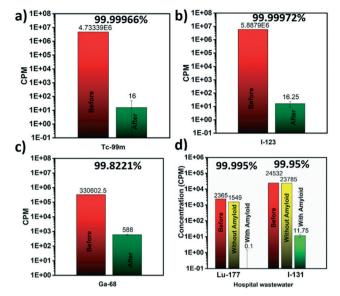
Fig. 2 Removal efficiencies for the different radioactive substances. Aqueous solutions filtrated by amyloid-carbon hybrid membranes using syringe aided setup for: (a) Tc-99m pertechnetate, (b) I-123, (c) Ga-68, and (d) hospital wastewater having the mixture of Lu-177 and I-131.
