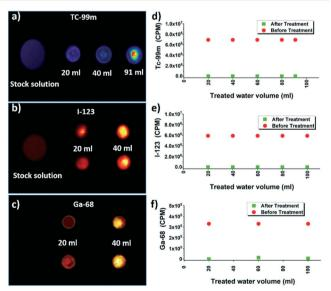
Fig. 3 Planar scintigraphy of: (a) Tc-99m, (b) I-123 and PET/CT images of (c) Ga-68 filters after filtration of different volumes of stock solution, with corresponding gamma counter measurements of the filtrate in (d)-(f), respectively.
