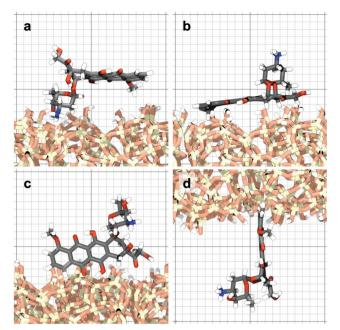
Fig. 4 Four representative configurations of the drug molecule adsorbed on the silica surfaces. The background grid has a cell size of 1 nm.
