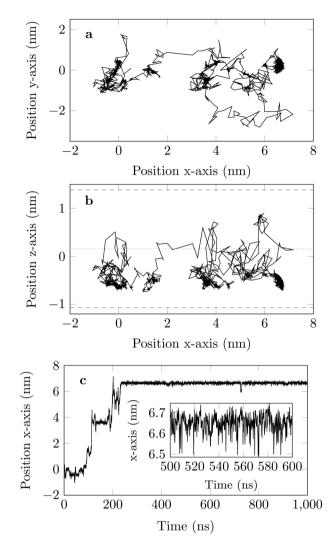
Fig. 5 One trajectory of the DOX molecule projected in the (a)  $\{x,y\}$ -plane and (b)  $\{x,z\}$ -plane recorded for 1000 ns, with COM positions shown every 200 ps. The averaged COM position of the hydrogen-surface atoms is the pair of grey dashed lines. The channel centre is the dotted line. Panel (c) shows the time evolution of the position along the x-axis.
