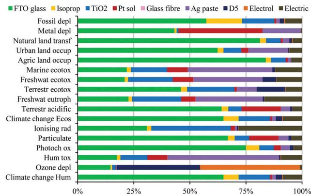
Fig. 4 Characterisation diagram of the environmental profile for the different device components in the manufacturing process of a virtual module with the organic D5 dye and  $I^-/I_3^-$  liquid electrolyte. Reproduced with permission from Elsevier.<sup>7</sup>
