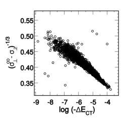
Fig. 1 A derived linear model relating the orthogonal component of the  $^1\text{H}$  shielding tensor in water  $(\sigma_\perp)$  to the stabilization energy due to charge-transfer ( $\Delta E_{\text{CT}}$ ). The shielding tensor component in the limit of a HB-free water molecule is denoted as  $\sigma_\perp^\infty$ . Reproduced from ref. 17/CC BY.
