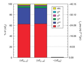
Fig. 2 Average contributions of the five strongest acceptor  $(\Delta E_{N \to C})$  and donor  $(\Delta E_{C \to N})$  interactions. The right-most column shows that higher-order delocalization does not significantly contribute to the overall binding (see also shaded areas in Fig. 5). Angular brackets within the axes labels denote averaging over all central water molecules and all AIMD snapshots. Reproduced from ref. 13.
