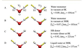
Fig. 11 The symmetric  $(\nu_1)$  and asymmetric  $(\nu_3)$  stretching modes of a water molecule and their splitting frequency  $\Delta\omega_{13}$  =  $\omega_3$  –  $\omega_1$  (A) in vacuum at 0 K, (B) in vacuum at 300 K, (C) of the H-bond donor of a water dimer at 0 K, and (D) in liquid water at 300 K, respectively. See eqn (7) for the definition of f<sub>d</sub>. Reprinted with permission from ref. 15. Copyright 2013 American Chemical Society
