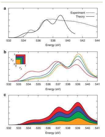
Fig. 8 XA spectra of liquid water. (a) Comparison of the calculated and experimental<sup>28</sup> XA spectra. (b) Calculated XA spectra of the four groups of molecules separated according to the asymmetry of their donor ( $\gamma_D$ ) and acceptor  $(\gamma_A)$  environments, as shown in the inset. (c) Contributions of the four groups into the total XA spectrum. The colour coding is shown in the inset above. Reproduced from ref. 13.
