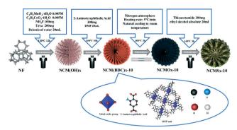
Scheme 1 Using NiCoMn(BDC)<sub>x</sub> as a precursor, an anion exchange method was used to synthesize highly disordered NCMS<sub>x</sub> compounds.
