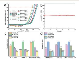
Fig. 7 (a) Polarization curves (iR-corrected) in the two-electrode configuration; (b) chronopotentiometry test of  $NCMS_{x-10}$  under overall water splitting; (c) comparison between the activities of different NCMO<sub>x</sub> materials in 1.0 M KOH; and (d) comparison between the activities of different NCMS<sub>x</sub> materials in 1.0 M KOH.
