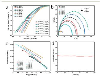
Fig. 5 (a) HER polarization curves (iR-corrected) obtained at a scan rate of 2 mV s $^{-1}$ ; (b) HER electrical impedance maps; (c) the Tafel slopes of the materials; and (d) results of the 100 h chronopotentiometry test of NCMS $_{\rm x}$  under HER.
