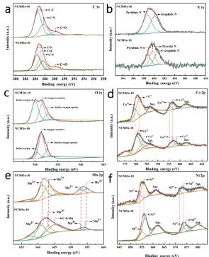
Fig. 3 (a-f) C 1s, N 1s, O 1s, Co 2p, Mn 2p, and Ni 2p spectra of  $NCMO_{x-10}$  and  $NCMS_{x-10}$ .
