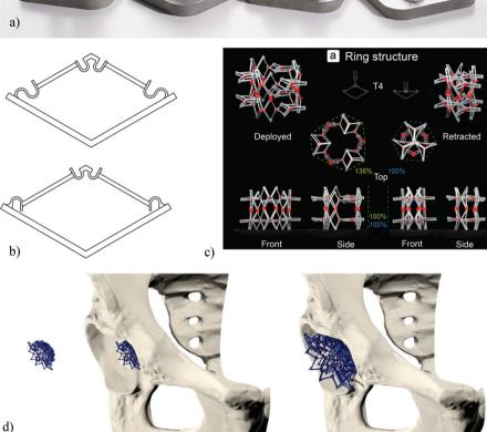
Fig. 1 (a) A number of AM orthopaedic implants (reprinted from ref. 46 with permission from Elsevier, Copyright 2018). (b) The basic bi-stable elements used for the design of multi-stable deployable implants.<sup>38</sup> (c) A deployable implant made through an arrangement of bi-stable implants.<sup>38</sup> (d) A schematic demonstration of the concept of deployable implants.<sup>38</sup>
