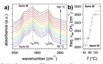
Fig. 6 (a) Evolution of the FTIR spectrum in the CH stretching area upon transition from the crystalline form IV to the lamellar phase III. (b) Position of the  $\nu_{\rm as} {\rm CH_2}$  band as a function of temperature.
