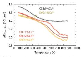
**Fig. 6** Variable temperature energy difference between the maxima of the  $^2F_{5/2}$  and  $^2F_{7/2}$  bands for YAG:2%  $Ce^{3+}$  (z=1, 2, and 3), CSS:1%  $Ce^{3+}$ , and SYG:1%  $Ce^{3+}$ , which are calculated from the fitting results shown in Fig. 2(b). Note that the results of SYG: $Ce^{3+}$  at the last two points (340 K and 360 K) appear to behave unexpectedly, which may be explained by the fitting errors due to relatively low intensity of the spectra (Fig. S1, ESI†).
