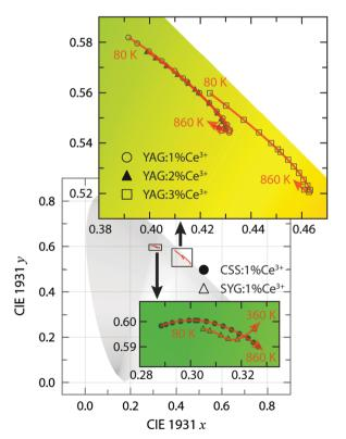
Fig. 3 Close-up views of the CIE 1931 color coordinate diagram for YAG:z%  $Ce^{3+}$  (z = 1, 2, and 3) in the green-yellow region, CSS:1%  $Ce^{3+}$ , and SYG:1% Ce3+ in the green region, upon excitation at 454 nm with varying temperature.
