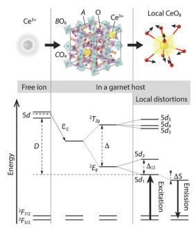
Fig. 1 Schematic illustration of the atomic environments (top) and energy level diagrams (bottom) of a free Ce<sup>3+</sup> ion, a Ce<sup>3+</sup>-doped garnet phosphor (a unit cell), and the local coordination of Ce<sup>3+</sup> in a garnet host.
