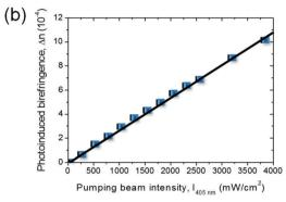
Fig. 3 Dependence of measured photoinduced birefringence on power excitation intensity from the pump beam (long-term photo-ordering). (a) Switching behaviour. (b) Dependence of the photoinduced refractive index anisotropy (birefringence), Δn, on the pumping beam intensity.
