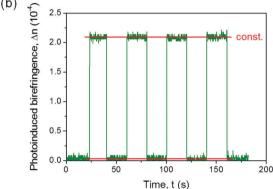
Fig. 4 (a)  $\Delta n$  values measured upon applied light modulation and (b) the multiple photoinduced birefringence process in PY-pCN/DNA-CTMA fibers ( $I_{pump} = 750 \text{ mW cm}^{-2}$ ).
