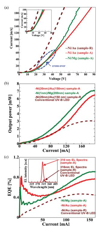
Fig. 5 UV-B LED sample-R with Ni/Au p-electrodes and sample-A both with Ni/Au and with Ni/Mg p-electrodes, measured at RT: (a) current vs. voltage (I-V) characteristics (the I-V characteristics under 100 mA is shown in the inset), (b) current vs. output power (I-L), and (c) current vs. EQE (I-EQE) characteristics under CW-operation under bare wafer conditions (wavelength vs. EL spectra are given in the inset).
