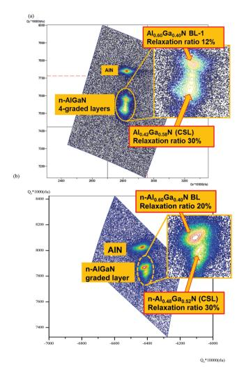
Fig. 3 (a) A reciprocal space map (RSM) for the (105) reflections of n-AlGaN CSL and graded BL, where strain-relaxation state and compositional information is shown in the inset of enlarged image (sample-A), and (b) a reciprocal space map (RSM) for the (105) reflections of n-AlGaN CSL and graded BL, where strain-relaxation state and compositional information is shown in the inset of enlarged image (sample-B).
