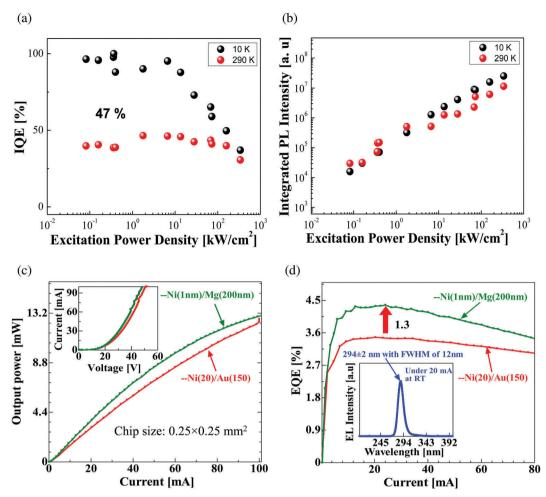
Fig. 6 (a) Excitation power density vs. IQEs measured at 10 K and 290 K for sample-B, and (b) temperature-dependence of PL as a function of excitation power density, (c) current vs. output power (I-L) (current vs. voltage (I-V) characteristics are given in the inset), and (d) current vs. EQE (I-EQE) characteristics of 294 nm UV-B LEDs with both Ni/Au and Ni/Mg p-electrodes under CW-operation under bare wafer conditions (sample-B) (wavelength vs. EL spectrum is given in the inset).
