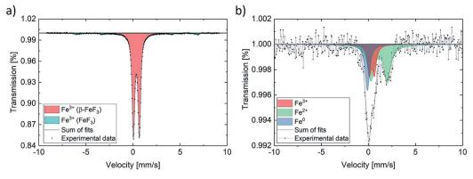
Fig. 4 Mössbauer spectrum for (a) as-prepared powder and (b) fully lithiated material (initial discharge).
