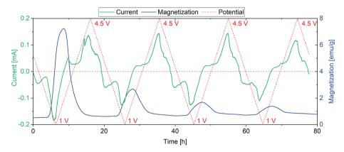
Fig. 2 Conversion reaction of  $FeF_3 \cdot 3H_2O$ . The sweep rate was set to 0.1 mV s<sup>-1</sup> to account for the slow kinetics of conversion reactions in general. Magnetization degradation with cycling is observed, reflecting the decreasing appearance of  $Fe^{(0)}$ .
