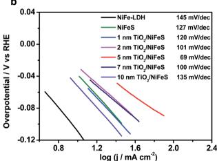
Fig. 2 Linear sweep voltammetry (LSV) curves (a) and the respective Tafel plots (b) of the ALD  $\rm TiO_2/NiFeS$  electrodes and  $\rm TiO_2/FTO$  (fluorine-doped tin oxide) electrodes measured in a 1 M KOH (aq) solution.
