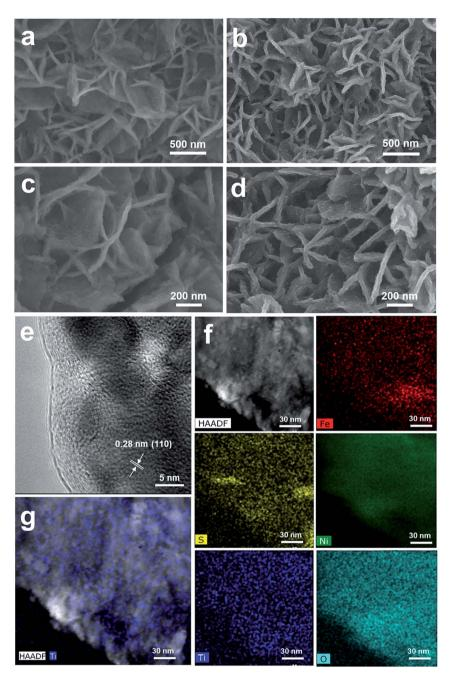
Fig. 3 Structural and elemental characterizations of the as-synthesized NiFeS (a and c) and 5 nm ALD  ${\rm TiO_2}$  grown on the NiFeS nanosheets by scanning electron microscopy (SEM) (b and d), and the high-resolution transmission electron microscopy (HRTEM) image (e), high-angle annual dark-field scanning transmission electron microscopy (HAADF-STEM) image, and energy dispersive X-ray spectroscopy (EDX) elemental mapping images of the 5 nm  ${\rm TiO_2/NiFeS}$  structure (f and q).
