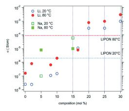
Fig. 10 Ionic conductivities for high entropy  $(MgCoNiCuZn)_{1-x-y}-Ga_yA_xO$  samples, where A=Li (circles) or Na (squares). The values usually observed for a LiPON solid conductor are also shown for comparison. Reproduced under the terms of the CC-BY 4.0 license. Copyright 2016, the authors, published by RSC Publishing.<sup>13</sup>
