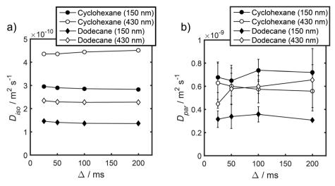
Fig. 6 (a)  $D_{\rm iso}$  and (b)  $D_{\rm par}$  values obtained by fitting APGSTE data to eqn (6). Macropore diameters are indicated in parentheses. Errors represent  $\pm 1$  standard deviation of three measurements of three different samples and are too small to be observed in (a).
