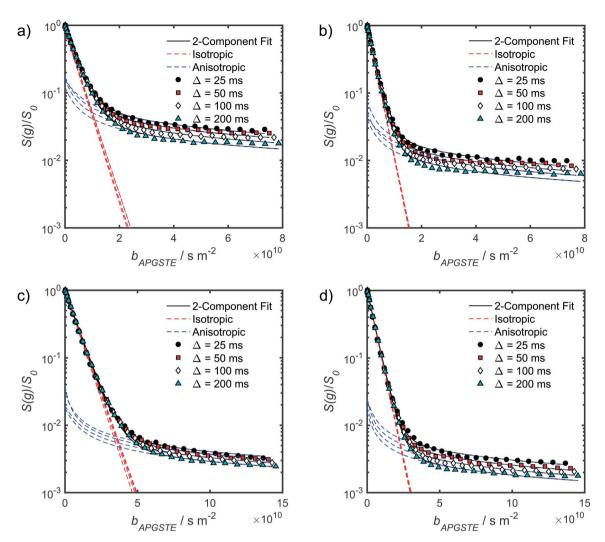
Fig. 5 APGSTE data for PrSO<sub>3</sub>H/MM-SBA-15 catalysts: PFG NMR signal attenuation curves for (a and b) cyclohexane saturated and (c and d) dodecane-saturated PrSO<sub>3</sub>H/MM-SBA-15 catalysts with respective 150 nm and 430 nm macropores. Two-component fits to the acquired data points utilised eqn (6); isotropic and anisotropic fitted components are shown in red and blue respectively.
