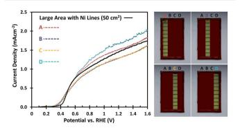
Fig. 4 AM1.5G J-V curves for the W:BiVO<sub>4</sub> photoanodes with Ni lines, measured on 4 different areas of the sample (right, A–D) to determine the uniformity of the photocurrent across the large area sample, with an electrolyte containing 0.5 M Na<sub>2</sub>SO<sub>3</sub> and 0.1 M KP<sub>i</sub> buffer of pH 7.
