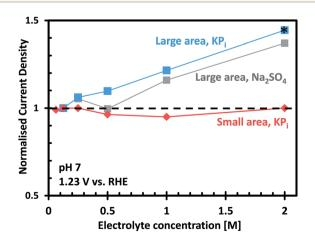
Fig. 6 Normalized photocurrent measured at  $1.23~V_{RHE}$ , under AM 1.5G illumination, for the small and large  $CoP_i/W:BiVO_4$  photoanodes as a function of concentration of electrolyte (pH 7). Zero concentration corresponds to pure deionized water. \*Electrolyte selected for all measurements using the large area  $BVO_4$  without hole scavenger.
