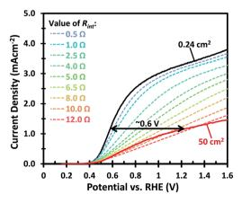
Fig. 2 The J-V curves of small (solid black) and large (solid red) W:BiVO<sub>4</sub> photoanodes measured in 0.5 M Na<sub>2</sub>SO<sub>3</sub> + 0.1 M KP<sub>i</sub> pH 7 buffer under AM 1.5G illumination. These curves are compared with the calculated J-V curves of a 50 cm<sup>2</sup> W:BiVO<sub>4</sub> photoanode (dashed lines) with the same performance as the small area sample, but subjected to different resistances from 0.5 to 12  $\Omega$ .
