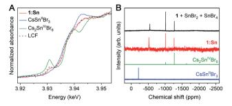
Fig. 2 (A) Sn  $L_3$ -edge XANES spectra of pulverized crystals of 1:Sn (1 atom% Sn) and  $CsSn^{II}Br_3$  and  $Cs_2Sn^{IV}Br_6$  standards. LCF denotes a linear combination fit of the two standards' spectra to that of 1:Sn. (B) <sup>119</sup>Sn NMR spectra of crystals of 1:Sn (1 atom% Sn),  $CsSn^{II}Br_3$ , and  $Cs_2Sn^{IV}Br_6$  dissolved in DMSO-d<sub>6</sub> and of 1 dissolved in DMSO-d<sub>6</sub> with  $SnBr_2$  and  $SnBr_4$  added to solution.
