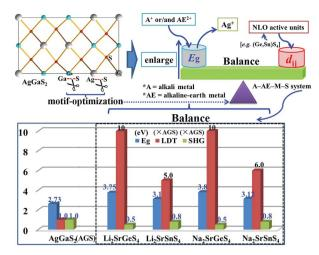
Fig. 6 Schematic diagram of designing new IR NLO materials by the motif-optimization with  $AgGaS_2$  as the template and title compounds achieve the suitable balance of wide  $E_q$  and good  $d_{ij}$ .
