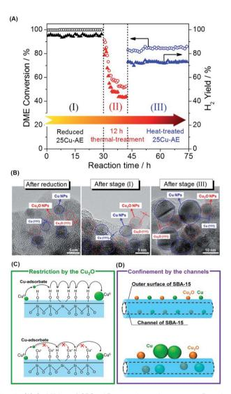
Fig. 3 (A) Stabilities of 25Cu-AE upon thermal treatment. Reaction conditions: (I) and (III): GHSV = 18 000 h $^{-1}$ , S/C = 2/1 (mol mol $^{-1}$ ),  $T=400\,^{\circ}\text{C}$ ; (II): GHSV = 36 000 h $^{-1}$ , S/C = 2/1 (mol mol $^{-1}$ ),  $T=450\,^{\circ}\text{C}$ ; (B) TEM images of 25Cu-AE during the stability test; (C) schematic representation of the restriction by the adjacent Cu<sub>2</sub>O; (D) schematic illustration of the spatial confinement by the channels.
