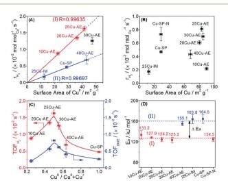
Fig. 4 Correlation of the H<sub>2</sub> production rate based on Cu<sup>0</sup> sites or total Cu sites with (A) the surface area of Cu<sup>0</sup> and (B) total surface area of Cu; (C) correlation of the TOF of  $H_2$  and DME with the  $Cu^0/(Cu^0 +$ Cu<sup>+</sup>) ratio; (D) apparent activation energies of the catalysts.
