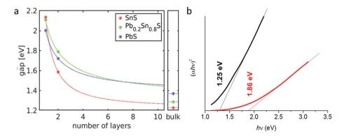
Fig. 10 Optical characterisation of  $Sn_{0.8}Pb_{0.2}S$ . (a) Calculated band gap energies of  $Sn_{0.8}Pb_{0.2}S$ , SnS, and layered PbS as a function of layer number. (b) Tauc plots of  $(\alpha h \nu)^2 vs. h \nu$  over the vis-NIR range of the electromagnetic spectrum, estimating direct optical band gaps of 1.25 eV for a standard  $Sn_{0.8}Pb_{0.2}S$  sol (black line) and 1.86 eV for the supernatant from a sol subjected to high speed centrifugation (11 600g, red line) respectively.
