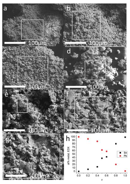
Fig. 3 Secondary electron SEM images (6 kV) of bulk  $Pb_{1-x}Sn_xS$  ( $0 \le x \le 1$ ) alloys. (a) x = 0 (i.e. PbS); (b) x = 0.2 (c), x = 0.4 (d) x = 0.5 (e) x = 0.6 (f) x = 0.8 (g) x = 1.0 (i.e. SnS). (h) at% of Sn and Pb found by EDX spectroscopy within the square areas of each image plotted as a function of compositional variation (x).
