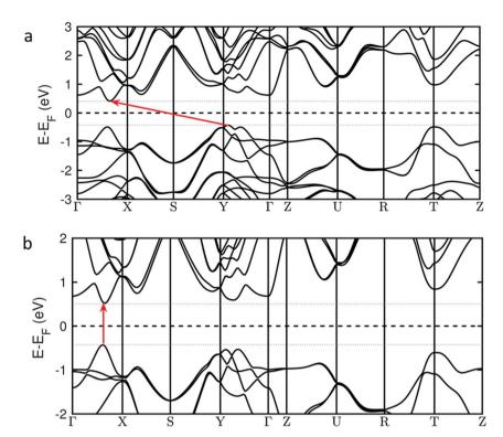
Fig. 11 Calculated band structures for bulk crystals of (a) SnS and (b) SnS in the  $Pb_{0.2}Sn_{0.8}S$  structure. The horizontal dashed lines show the Fermi energies and the red arrows the HOCO-LUCO excitations. HOCO (highest occupied crystal orbital) and LUCO (lowest unoccupied crystal orbital) are the edges of the valence and conduction bands respectively. The Fermi energy is set to zero
