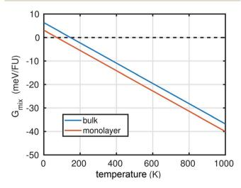
Fig. 5 Calculated thermodynamic stability of Pb $_{0.2}$ Sn $_{0.8}$ S alloy. Plot of the Gibbs free energy of mixing  $G_{\rm mix}$  for a Pb $_{0.2}$ Sn $_{0.8}$ S alloy versus temperature in kelvins as calculated by a thermodynamic model in bulk and in monolayer. The result suggests that mixing of PbS and SnS is unfavourable at T=0 K, but at the temperature of synthesis of the bulk alloys (723 K) and room temperature (298 K), mixing is thermodynamically favourable.
