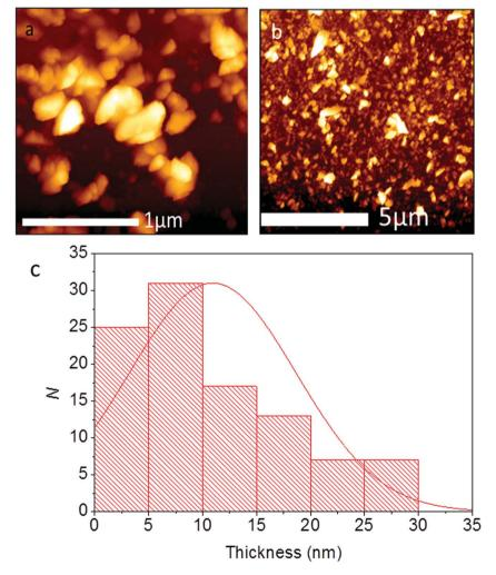
Fig. 8 AFM analysis of Pb<sub>0.2</sub>Sn<sub>0.8</sub>S nanosheets (N=100). (a) High magnification height image of Pb<sub>0.2</sub>Sn<sub>0.8</sub>S nanosheets. (b) Low magnification AFM height of Pb<sub>0.2</sub>Sn<sub>0.8</sub>S nanosheets. (c) Histogram of thicknesses of Pb<sub>0.2</sub>Sn<sub>0.8</sub>S sheets with a normal distribution overlayed ( $\bar{x}\pm\sigma=10.9\pm7.7$  nm).
