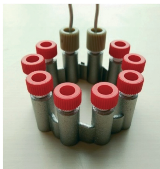
Fig. 6 3D printed CSTR cascade (AP01) closed with standard HPLC fittings. The 3D printed 10–32 UNF thread had to be refined after printing.
