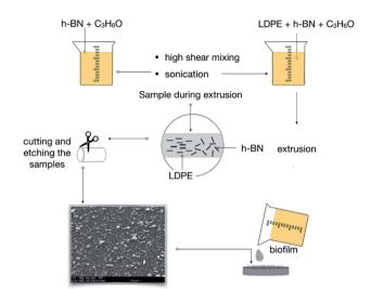
Fig. 1 The scheme of preparation and extrusion of BN-LDPE composites with the vertically oriented BN nanoflakes on the surface.
