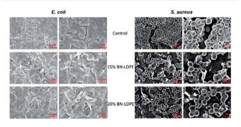
Fig. 4 Representative SEM images of *E. coli* and *S. aureus*. *E. coli* and *S. aureus* were grown for 24 h on LDPE (control) and LDPE composites with 15 and 20% of BN-LDPE composites and grown bacterial cells were fixed and dehydrated before SEM imaging.
