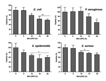
Fig. 3 Measurement of bactericidal activity extruded LDPE composites with 0–20% of BN after the 24 h of bacterial growth. Results are presented as a mean  $\pm$  standard deviation error of viability percentage of each bacterial strains in compared to control. \*P < 0.005, \*\*P < 0.001.
