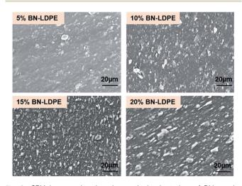
Fig. 2 SEM images showing the vertical orientation of BN on the extruded BN-LDPE composites with 5-20% of BN.
