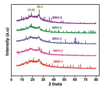
Fig. 9 WAXRD spectra of the as-prepared MRHs.
