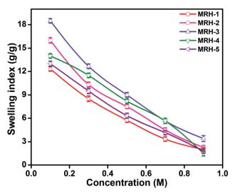
Fig. 7 Swelling indices of the as-prepared MRHs in CaCl<sub>2</sub> solutions.
