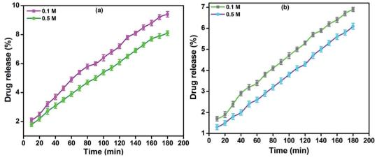
Fig. 15 Drug release profiles of MRH-3 in (a) NaCl and (b) CaCl<sub>2</sub> solutions.
