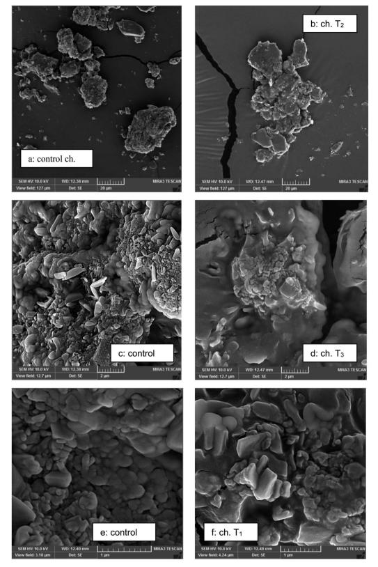
Fig. 2 Particle agglomeration of chocolates sweetened with sucrose and polyols obtained with scanning electron microscopy: (a, c and e) control chocolates; (b, d and f) sucrose-free chocolates.
