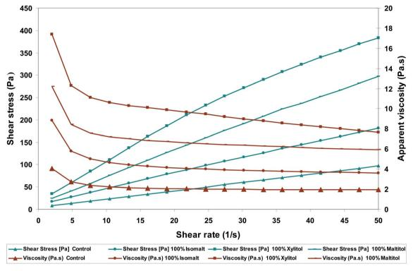
Fig. 1 Effects of sugar replacers on shear stress and apparent viscosity-shear rate rheograms of functional milk chocolates
