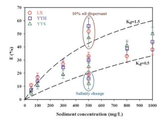
Fig. 5 Modeling of predicting the submerged oils formation as a function of sediment concentrations. The dash lines represent the model results computed using eqn (7) based on  $K_{\rm d}=0.5$  and 1.5 mL mg<sup>-1</sup>. Note: The use of chemical dispersant and change of salinity lead to deviate from model results.
