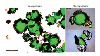
Fig. 2 Submerged oils formed observed by UV epi-fluorescence. Fluorescing green indicates the oil droplets.
