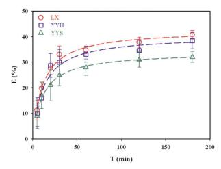
Fig. 4 The kinetics of submerged oil formation for the three test oils. Note: the dashed lines are fitted by eqn (4).
