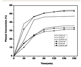
Fig. 13 Evolution of phenol conversion during single run catalytic tests for CuCe oxi  $(\triangle)$ , CuCe red  $(\blacktriangle)$ , CuAl oxi  $(\bigcirc)$ , CuAl red  $(\blacksquare)$ , CuAlCe oxi  $(\square)$ , CuAlCe red  $(\blacksquare)$ .
