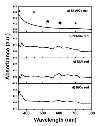
Fig. 6 Spectra UV-Vis for the calcined Ni supported catalyst: (a) and for the reduced Ni supported catalysts: (b), (c) and (d). Legend: (#) Ni<sup>+2</sup> (Td), (\*) Ni<sup>+2</sup> (Oh).
