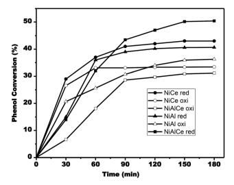
Fig. 15 Evolution of phenol conversion during single run catalytic tests for NiAlCe oxi ( $\square$ ), NiAlCe red ( $\blacksquare$ ), NiAl oxi ( $\triangle$ ), NiAl red ( $\blacktriangle$ ), NiCe oxi ( $\bigcirc$ ), NiCe red ( $\blacksquare$ ).
