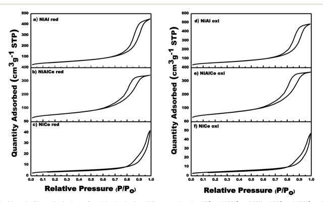
Fig. 2 Adsorption/desorption isotherms for calcined and reduced Ni supported catalyst: NiCe oxi, NiAlCe oxi, NiAlCe oxi, NiAl oxi, NiCe red, NiAlCe red and NiAl red.
