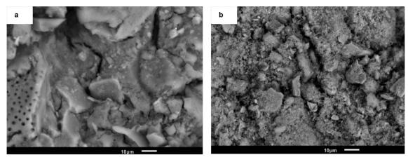
Fig. 9 SEM images for (a) NiAl red and (b) NiCe red, with  $\times 1000$
