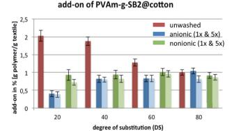
Fig. 3 Quantitative determination of the add-on of PVAm-g-SB2 on PET and cotton by ICP-OES. After the finishing step, textiles were thoroughly rinsed with water (no detergent, red columns) and subsequently washed either with anionic (blue columns) or nonionic (green columns) detergents. Number of wash cycles:  $1\times$  (dark),  $5\times$ (pale).
