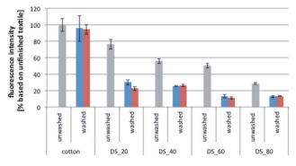
Fig. 5 Results of the protein adhesion tests for different fabrics (PET and cotton). The fabrics were finished with sulfobetaine-modified PVAm-g-SB2 with different degrees of substitution (DS) and then used either directly after rinsing with water (unwashed) or after 1 wash cycle (blue columns) and 5 wash cycles (red columns) according to DIN EN ISO 105-C06 using ECE detergent.
