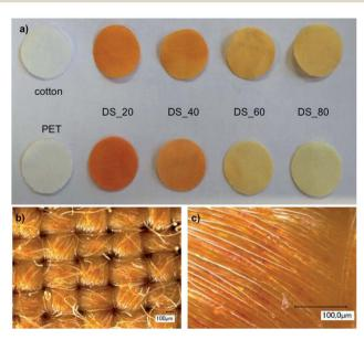
Fig. 2 Characterization of the polymer add-on: (a) photographs of textiles (cotton and PET) finished with PVAm-g-SB2 with varying DS that were stained by TNBS; (b) and (c) light microscopic pictures of PET finished with PVAm-q-SB2\_20 after TNBS staining
