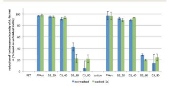
Fig. 9 Antibacterial activity before and after 5 wash cycles against the Gram-negative strain A. fischeri of different PET and cotton fabrics modified with PVAmg-SB2 with different DS
