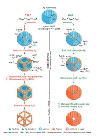
Fig. 7 Schematic illustration describing the mechanisms proposed for the deposition of Au and Ag atoms on Ag NCs when HAuCl<sub>4</sub> is titrated into an agueous suspension of Ag NCs in the presence of H<sub>2</sub>Asc, NaOH, and CTAC (left) or PVP (right) at an initial pH of 11.6. Adapted with permission from ref. 101. Copyright 2017, American Chemical Society.
