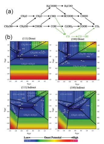
Fig. 16 (a) Schematic representation of the reaction pathways and possible intermediates considered here for methanol electrooxidation. Green arrows indicate the indirect mechanism to CO<sub>2</sub> formation. (b) Potential-determining steps for methanol electrooxidation on (111) and (100) facets plotted using  $G_{CO^*}$  and  $G_{OH^*}$  as the descriptors. Adapted with permission from ref. 190. Copyright 2009, American Chemical Society.
