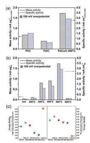
Fig. 12 (a) and (b) Comparison of HOR mass and specific activity (MA and SA) of Pt/C, Pd/C, and PdCu/C at overpotential of 100 mV in H2saturated 0.1 M KOH electrolyte. (c) Equilibrium adsorption potentials (vs. RHE) for \*H (1/6 ML) and \*OH (1/3 ML) on Pt, Pd, bcc-PdCu (B2 phase), and fcc-PdCu (L1<sub>0</sub> and B13 phases) terrace surfaces. The three PdCu surfaces shown here are covered by 1 mL Pd. Adapted with permission from ref. 148. Copyright 2018, Royal Society of Chemistry.
