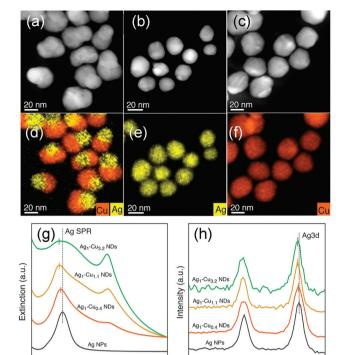
Fig. 25 (a-c) HAADF-STEM images of Aq1-Cu1.1 NDs (a), Aq NPs (b), and Cu NPs (c); (d-f) corresponding EDX elemental maps of Cu (orange) and Ag (yellow) of Ag1-Cu1.1 NDs (d), Ag NPs (e), and Cu NPs (f). (g) UV-vis spectra and (h) XPS spectra of Ag/Cu nanocrystals. Adapted with permission from ref. 279. Copyright 2019, American Chemical Society.
