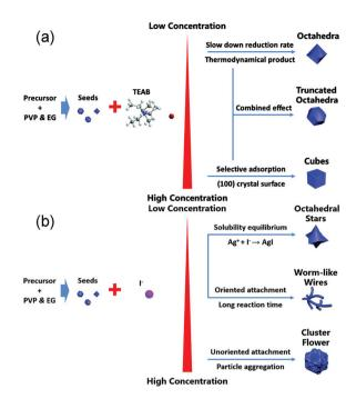
Fig. 4 Synthesis pathways of (a) single-crystalline Pt-Ir alloy nanocrystals and (b) polycrystalline Pt-Ir alloy nanocrystals. Adapted with permission from ref. 62. Copyright 2017, Royal Society of Chemistry.
