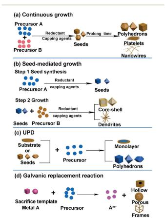
Fig. 2 General strategies used in shape-controlled synthesis of noblemetal-based nanostructures. (a) Continuous growth. (b) Seed-mediated growth. (c) UPD. (d) Galvanic replacement reaction.
