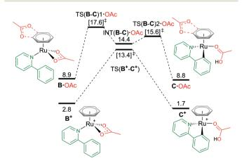
Fig. 4 BP86-D3BJ(BS2.MeCN)//BP86(BS1) free energy values 120 °C for C-H activation of a-H in species B+ and B-OAc relative to A,  $[(C_6H_6)Ru(OAc)_2]$ , in kcal mol<sup>-1</sup>.
