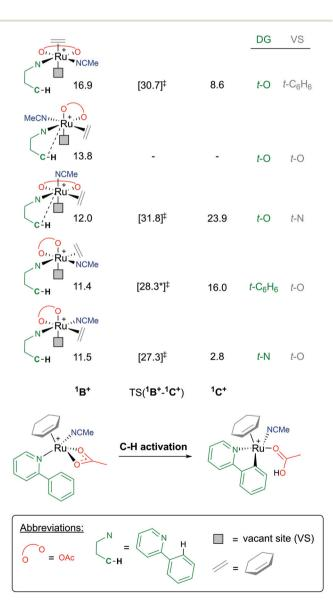
Fig. 8 BP86-D3BJ(BS2,MeCN)//BP86(BS1) free energy values at 120 °C for C-H activation of a-H for isomers of <sup>1</sup>B<sup>+</sup>, relative to A, [(C<sub>6</sub>H<sub>6</sub>)Ru  $(OAc)_2$ , in kcal  $mol^{-1}$
