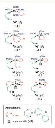
Fig. 9 BP86-D3BJ(BS2,MeCN)//BP86(BS1) free energy values at 120 °C for isomers of G, relative to A,  $[(C_6H_6)Ru(OAc)_2]$ , in kcal  $mol^{-1}$  {chemdraws of each isomer do not necessarily represent the most stable intermediate energy quoted, but are to highlight the differences in each "G" species).
