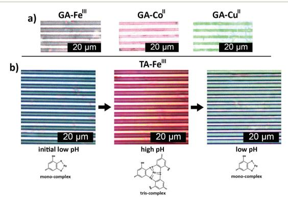
Fig. 4 Tuning the color of hydrolyzable tannin-metal ion nanoparticles patterned on CNF films. (a) Optical images of GA-impregnated CNF films patterned with Fe<sup>III</sup>, Co<sup>II</sup> and Cu<sup>II</sup> ion salt solutions. (b) pH-Dependent reversible color change and stoichiometry of TA-Fe<sup>III</sup> complexes patterned on CNF film.
