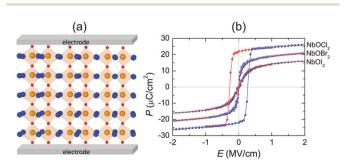
Fig. 8 Electrostatic energy storage in a 2D FE capacitor. (a) Schematic model for a 2D FE capacitor device based on NbOX<sub>2</sub> monolayers. (b) MC simulated P-E loops for NbOX<sub>2</sub> monolayers at room temperature. Electric field E is applied along the polar axis. Results corresponding to the electric charging and discharging processes are marked in red and blue colors, respectively.
