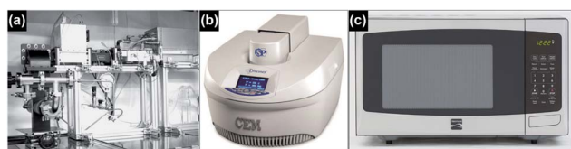
Fig. 6 Schematic illustration of (a) the single-mode microwave system, reproduced from ref. 38, with permission from Elsevier, 2006; (b) laboratory microwave oven, reproduced from ref. 56, under the license of CC BY 4.0; and (c) domestic microwave oven, reproduced from ref. 57, under the license of CC BY 4.0.
