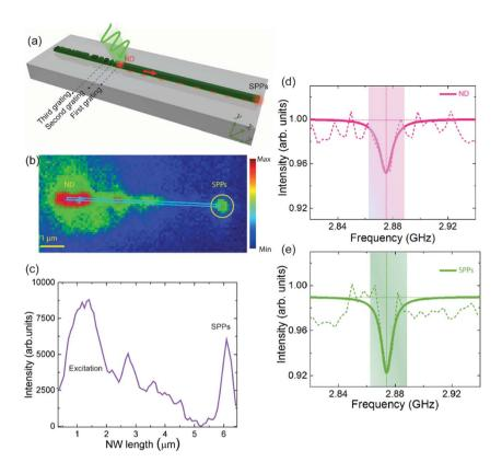
Fig. 3 (a) Schematic of the NW-OGC system based on a MPTMS adhesion layer coupled to the NV centre in NDs showing a map of the variable displacement of the ND. The corresponding photon emission map and intensity profile are shown in (b and c), respectively. Measurement of the NV spin state readout in a ND coupled NW-OGC system showing a reduction in the photoluminescence intensity in ND emission (d) and a reduction in the SPP scattering strength (e).
