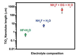
Fig. 3 Effect of the electrolyte composition on the length of titania nanotubes formed during anodization.
