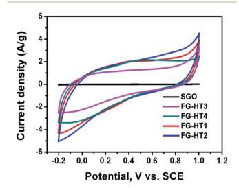
Fig. 11 Cyclic voltammograms of spongy graphene oxide and hydrogenated  ${\rm TiO_2}$  with different ratios of functionalized graphene oxide. Reproduced from ref. 117 with permission from the Royal Society of Chemistry.
