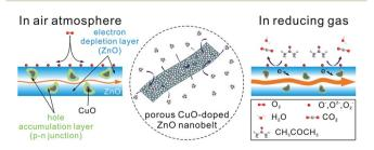
Fig. 8 Possible enhanced sensing mechanism for porous CuO-doped ZnO nanobelts
