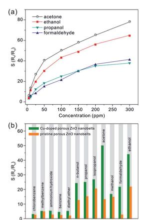
Fig. 7 (a) The relationship between the relative response and the concentration of some typical VOCs (acetone, ethanol, propanol, and formaldehyde), and (b) the relative responses of CZ-3 porous nanobelts toward all investigated VOCs (100 ppm) in contrast to those of pristine porous ZnO nanobelts at the optimal working temperature of 325 °C
