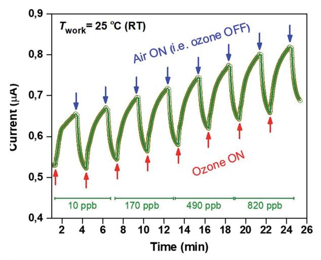
Current changes at room temperature of Cu<sub>2</sub>O nanocubes due to successive increases in O<sub>3</sub> concentrations.
