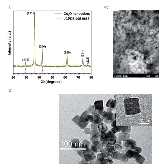
Fig. 2 (a) X-ray diffraction (XRD) pattern of Cu<sub>2</sub>O nanocubes and standard Cu<sub>2</sub>O card. (b and c) FESEM images and TEM images of Cu<sub>2</sub>O nanocubes.
