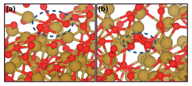
Fig. 7 Top views of  $O_3$  species over a (001)  $Cu_2O$  surface: (a) a chemisorbed  $O_3$  protrusion (dashed line) with one Cu-O bond. (b) An  $O_3$ -related bridge (dashed line) between surface Cu atoms. The  $O_3$  moiety forms three O-Cu bonds. (Cu: brown, O: red spheres).
