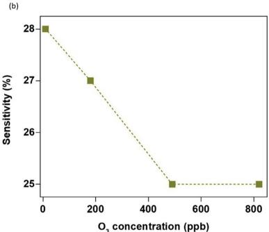
Fig. 5 (a) Response and recovery time (s) of the sensor at different ozone concentrations. (b) Sensing sensitivity as a function of ozone concentration.
