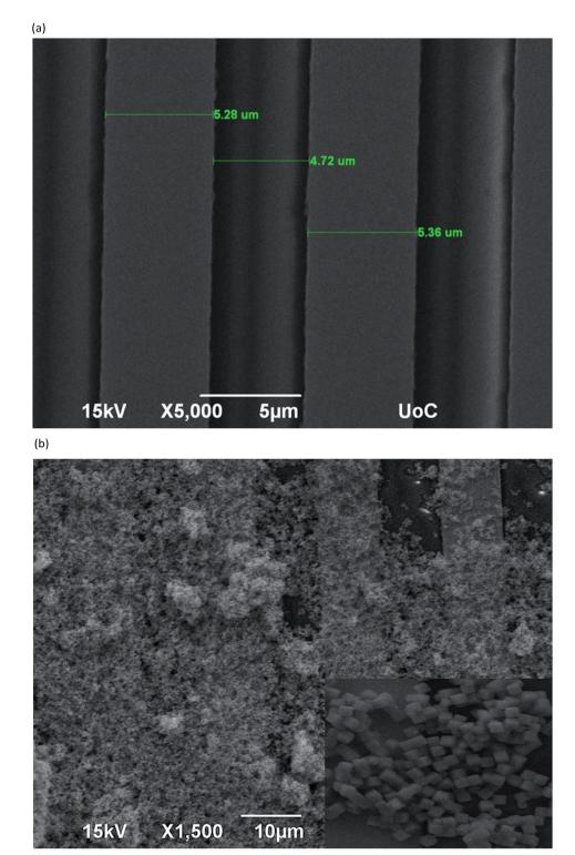
Fig. 3 (a) SEM images of the IDEs with a gap of 5 μm. (b) SEM of coated IDEs and zoomed view of the coated IDEs with nanocubes in the inset.
