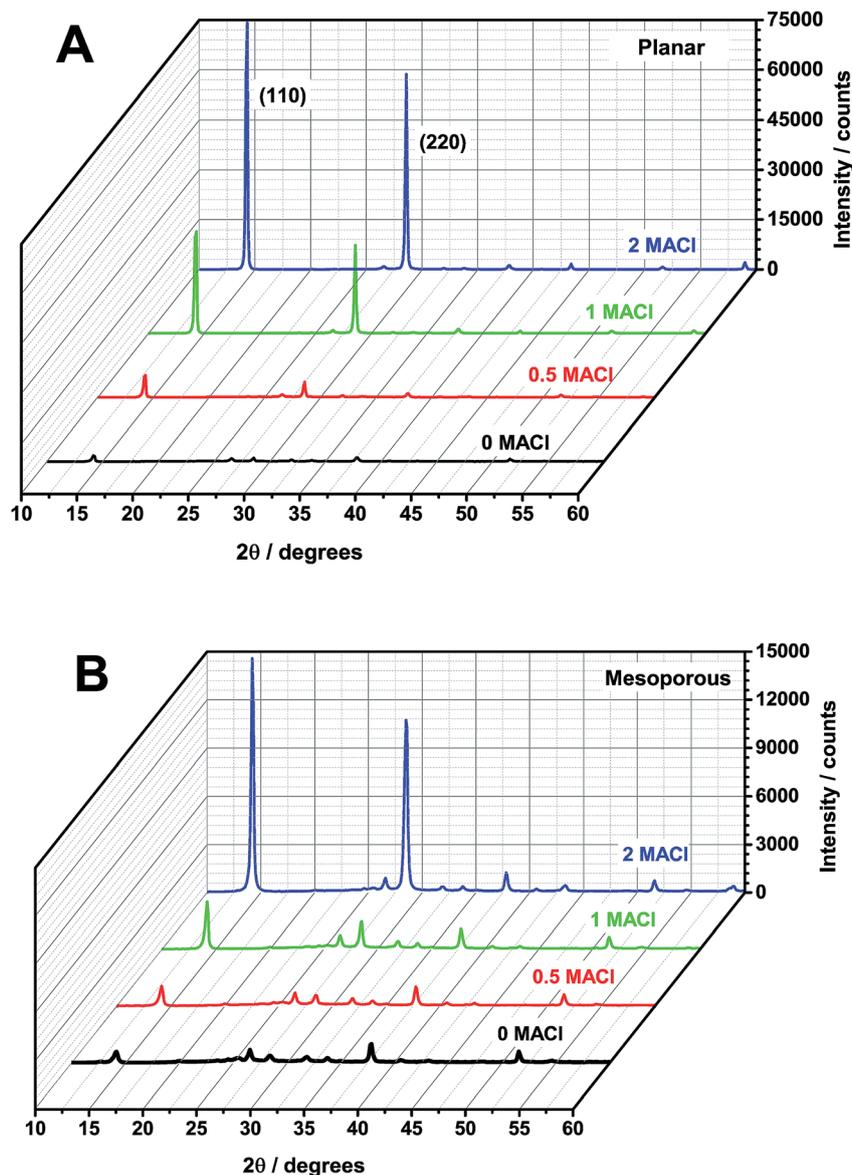
Fig. 1 XRD of the perovskite films with 0 MACI (black), 0.5 MACI (red), 1 MACI (green), and 2 MACI (blue) precursor ratios coated on (A) planar and (B) mesoporous titania. The (110) and (220) peaks are labeled here and all peaks are further indexed in Fig. S1.†
