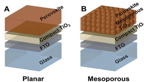
Scheme 1 Illustration of the sample architectures studied in this work. (A) “Planar” architecture consisting of perovskite/planar  $\text{TiO}_2$ /FTO and (B) the “mesoporous” architecture consisting of perovskite/mesoporous  $\text{TiO}_2$ /planar  $\text{TiO}_2$ /FTO.
