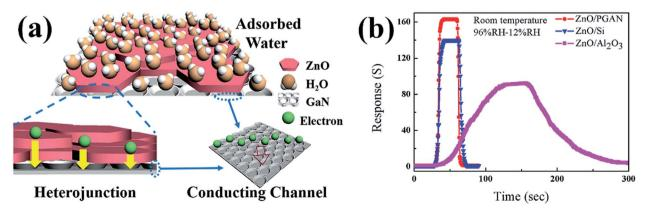
Fig. 6 (a) Schematic of  $H_2O$  molecule interaction with the ZnO/PGAN HS. Electron transport on the ZnO/PGAN heterojunction (bottom-left) and effective electron transport on GaN (bottom-right). (b) Response curves of humidity sensors based on ZnO/PGAN, ZnO/Si and ZnO/Al<sub>2</sub>O<sub>3</sub>.
