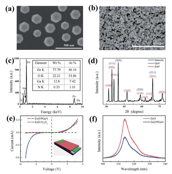
Fig. 3 (a) SEM image of ZnO disks on silicon wafer. (b) SEM image of ZnO disks sprayed on PGAN. (c) EDS analysis results for all the area of the material in (b). (d) XRD pattern of ZnO/PGAN. (e) I-V characteristics of the ZnO/PGAN heterojunction and ZnO/Al<sub>2</sub>O<sub>3</sub> samples measured at room temperature exposed to atmosphere. (f) Photoluminescence spectra of pristine ZnO and ZnO/PGAN heterojunctions
