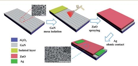
Fig. 1 Schematic illustration of the fabrication process of ZnO/PGAN humidity sensors.
