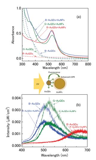
Fig. 1 (a) UV-vis absorption spectra and (b) fluorescence spectra of AuQDs and AuQD:AuNP aqueous solution.
