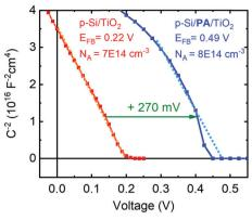
Fig. 5 Mott-Schottky analysis of p-Si/TiO<sub>2</sub> and p-Si/Al<sub>2</sub>O<sub>3</sub>/PA/TiO<sub>2</sub> PV cells obtained from impedance measurements in the dark. Experimental and fitting details are given in the ESI.† The measured doping densities match with the resistivity data provided by the manufacturer.
