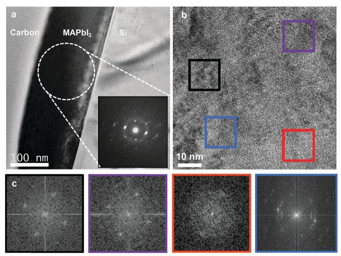
Fig. 4 TEM electron diffraction analysis of MAPbl<sub>3</sub> perovskite grains. (a) Cross-section image of single perovskite grain on Si(100) substrate and selected area electron diffraction (SAED) pattern collected from the region indicated (inset). (b) Higher-magnification TEM and (c) fast Fourier transform (FFT) patterns generated across different regions of the grain shown in (b)
