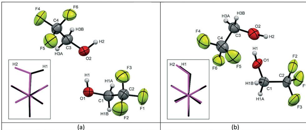
**Fig. 1** The labelling schemes used in the crystal structures of TFE for (a) the low temperature form 1 and (b) the high pressure form 2, with thermal ellipsoids drawn at the 50% probability level. The inserted images show the molecular overlay $\ddagger$  of the two independent molecules in the asymmetric unit with molecule 1 (O1, C1, C2, F1, F2, F3) shown in black and molecule 2 (O2, C3, C4, F4, F5, F6) shown in pink (C – dark grey, H – light grey, O – red, F – green).
