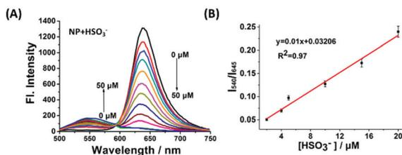
Fig. 1 (A) The fluorescence responses of 10  $\mu\text{M}$  NP upon addition of NaHSO<sub>3</sub> (0–50  $\mu\text{M}$ ).  $\lambda_{\text{ex}} = 446 \text{ nm}$ . (B) The relationship between fluorescence ratio ( $I_{540}/I_{645}$ ) and  $[\text{HSO}_3^-]$ .
