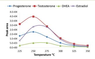
**Fig. 2** Effect of the CPI temperature on SRM peak areas of steroids from a standard solution 100 ng mL<sup>-1</sup>.
