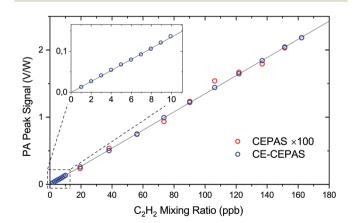
Fig. 5 CE-CEPAS and CEPAS 2<sup>nd</sup> harmonic peak values as a function of the target gas mixing ratio.
