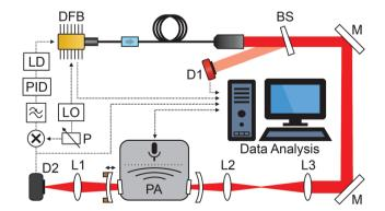
Fig. 1 Schematic picture of the CE-CEPAS instrument. DFB: distributed feedback laser, BS: beam sampler, M: mirror, LD: laser driver, PID: feedback controller, LO: local-oscillator, P: phase control, D: photodetector, L: lens, PA: photo-acoustic analyser.
