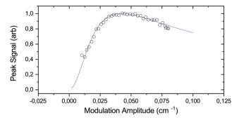
Fig. 4 Measured and simulated photo-acoustic 2<sup>nd</sup> harmonic peak signal levels for a  $C_2H_2$  line at 200 mbar.
