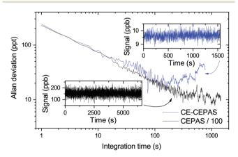
Fig. 6 Allan deviation of the  $2^{nd}$  harmonic peak values of CE-CEPAS and CEPAS in the case of a small amount of the target gas  $(C_2H_2)$ . CEPAS values have been divided by the enhancement factor BUF = 100 for comparison.
