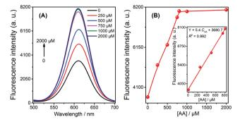
Fig. 3 The analytical performance of this ascorbic acid sensor in 1% fruit juice solution. (A) Fluorescence emission spectra of the biosensor upon the addition of different concentrations of AA. (B) Calibration curve with the inset showing the linear relationship of the fluorescence signal *versus* the concentration of AA ranging from 0.5 to 800  $\mu$ M. Error bars were estimated from three replicate measurements.
