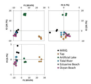
Fig. 6 LDA score plot for the analysis of Cu<sup>2+</sup> (100 μM) doped environmental water samples performed in quintuplicate (pH 7.4, 20 mM HEPES). Each pairing of the three main factors is plotted in a separate 2D plot.
