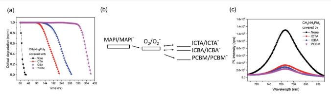
Fig. 3 (a) Normalized optical degradation of CH<sub>3</sub>NH<sub>3</sub>Pbl<sub>3</sub> with the coverage of ICTA, ICBA and PCBM films. (b) Suggested mechanism of electron transfer from superoxide to fullerene derivative acceptors. CH<sub>3</sub>NH<sub>3</sub>PbI<sub>3</sub> is represented as MAPI. (c) Photoluminescence of CH<sub>3</sub>NH<sub>3</sub>PbI<sub>3</sub> films covered with ICTA, ICBA and PCBM under 1 sun in N2.
