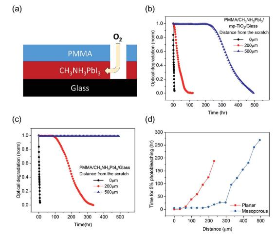
Fig. 5 (a) Illustration of oxygen diffusion in the scratched  $CH_3NH_3PbI_3/PMMA$  film. Normalized optical degradation of  $CH_3NH_3PbI_3$  at different distances from the scratch on (b) a mesoporous  $TiO_2$  scaffold substrate and (c) a planar substrate. (d) The distance from the scratch for 5% photobleaching of  $CH_3NH_3PbI_3$  versus time on planar/mesoporous substrates. The measurements were done in dry air and under 1 sun LED illumination.
